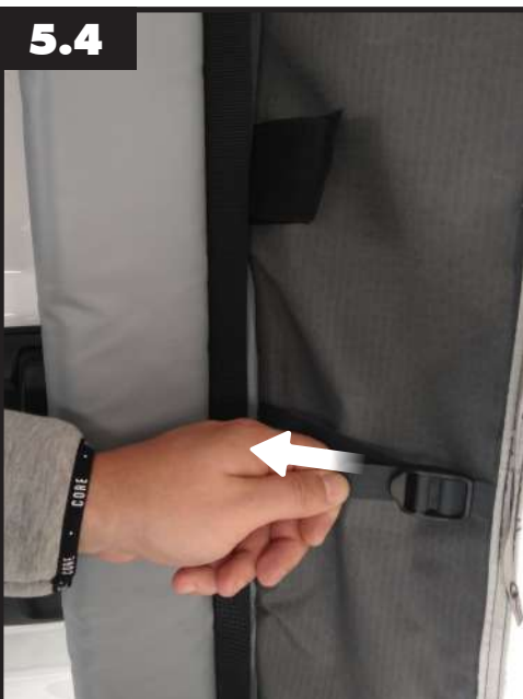
Tigh straps on the inside to compress the side panel. We will have an optimal adaption to the van profile.
